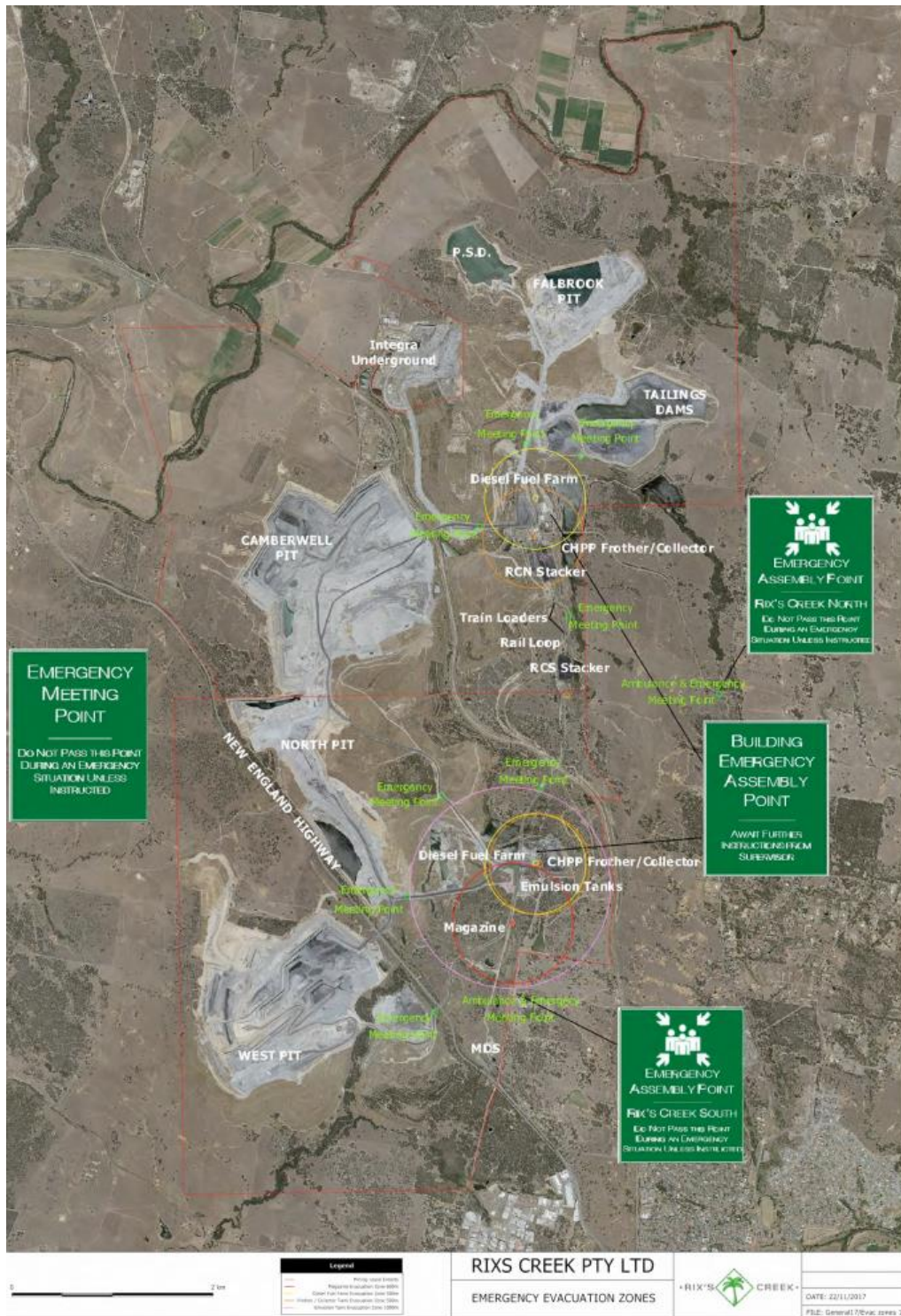
Figure 7 Rix's Creek Emergency Evacuation Plan and Location of Bulk Flammable Liquids and Materials
