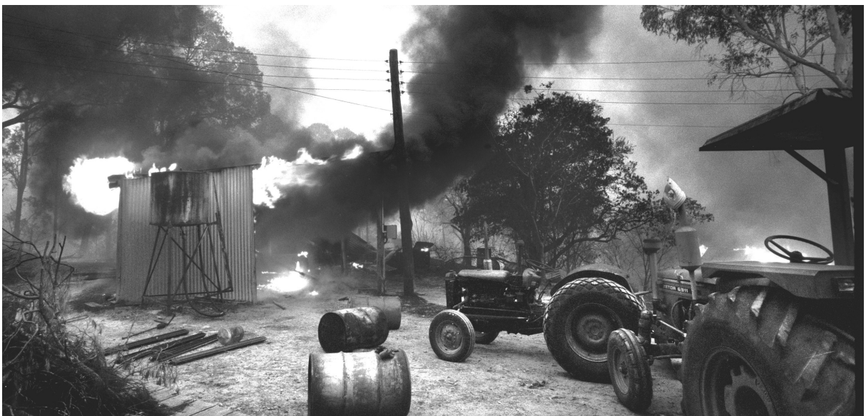
Class 10a buildings such as sheds should be located >10 metres from a building of another class unless they also comply with the relevant construction requirement of the main building under AS 3959 - 1999 and the BCA.
