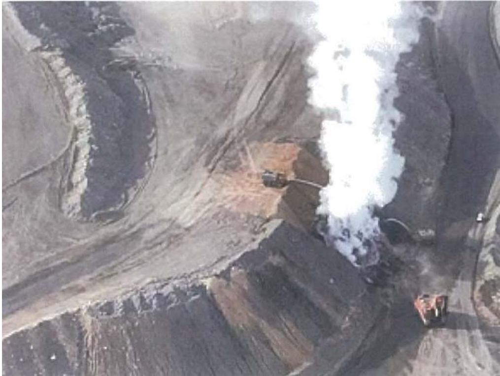
Photo 1: Showing "hot spot" in dump being controlled (source: DRG Severe Incident Report, 2018)
