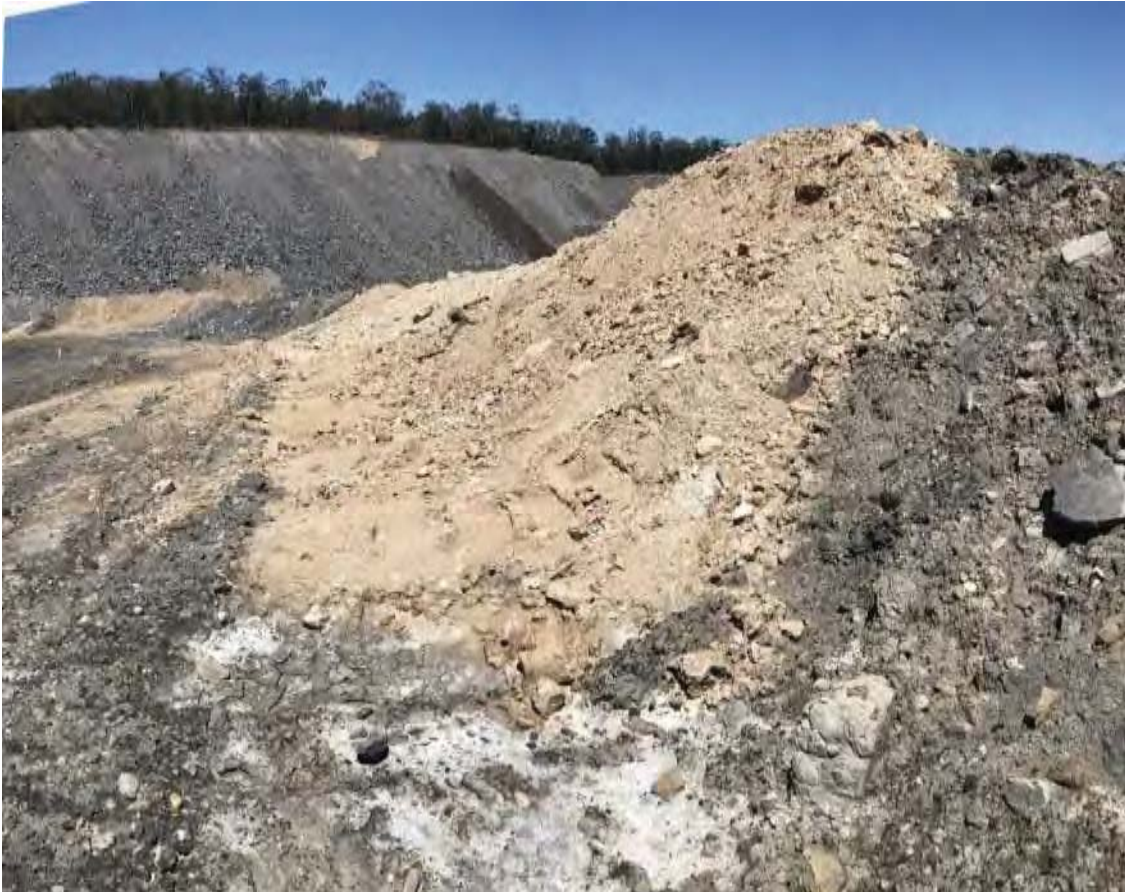
Photo 7: Covering of clay over spontaneous combustion area
