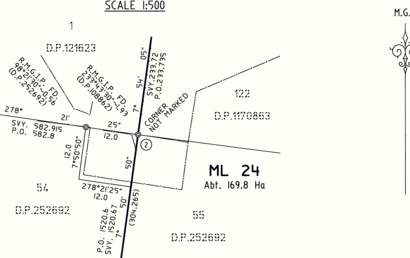
RTK GNSS OBSERVATIONS WERE USED TO DERIVE PARTS OF THIS SURVEY
