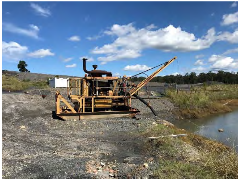
Photo 2 - Diesel pump installed at overland dam.
