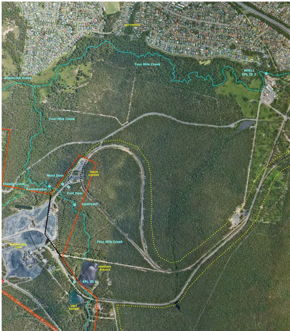
Figure 1. Plan showing sediment dam, Licenced discharge point (EPA ID1) and sampling locations in relation to Project Approval, EPL and Mining Tenements.
