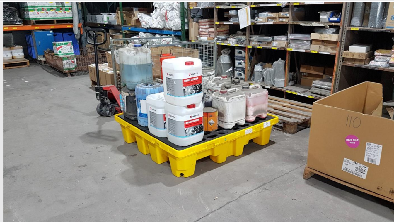
Plate 3 Oil and chemical storage in bunding inside a storage shed
