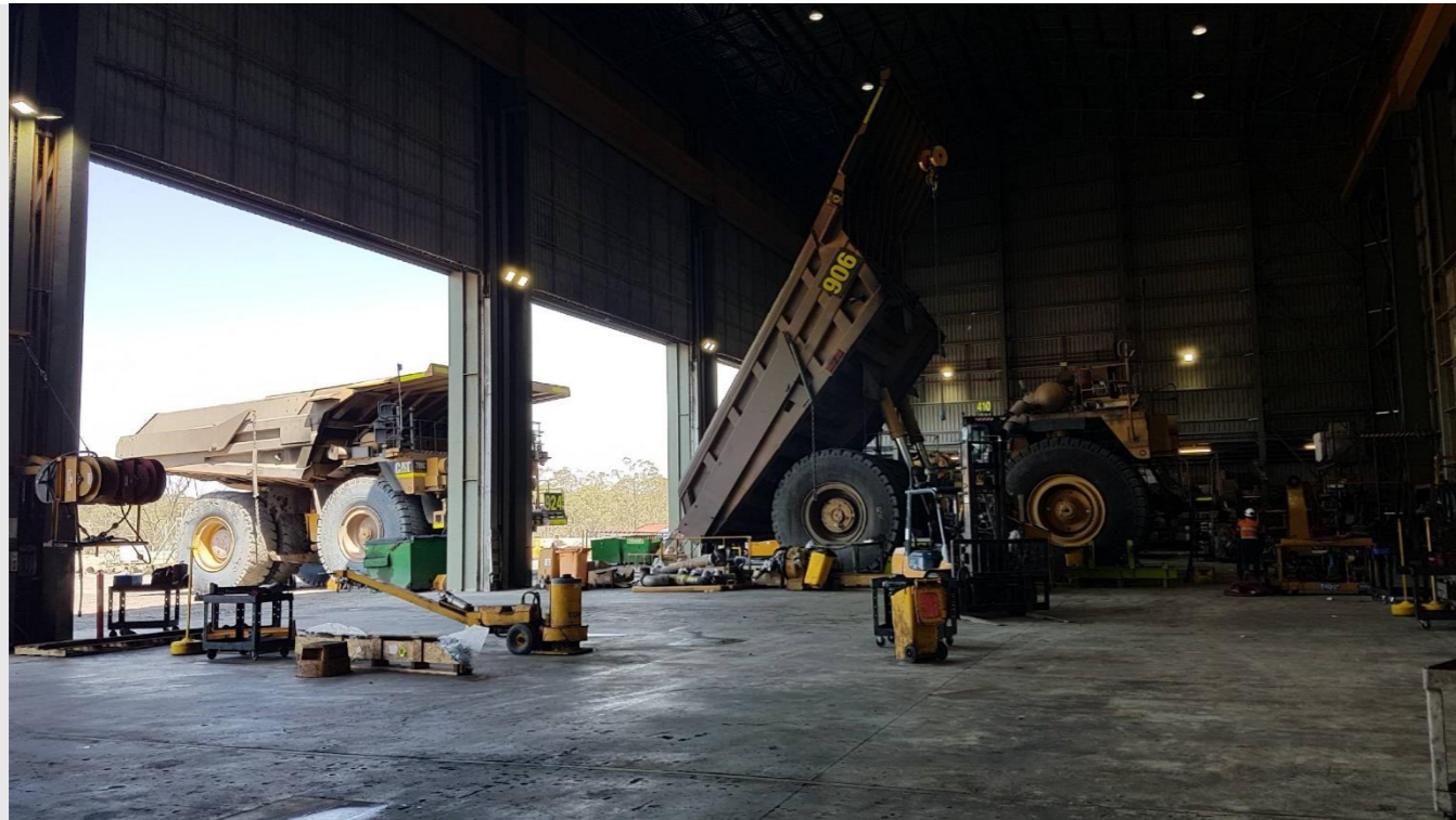
Plate 10 Maintenance works within the bunded workshop Draining to the oil/water separation system.
