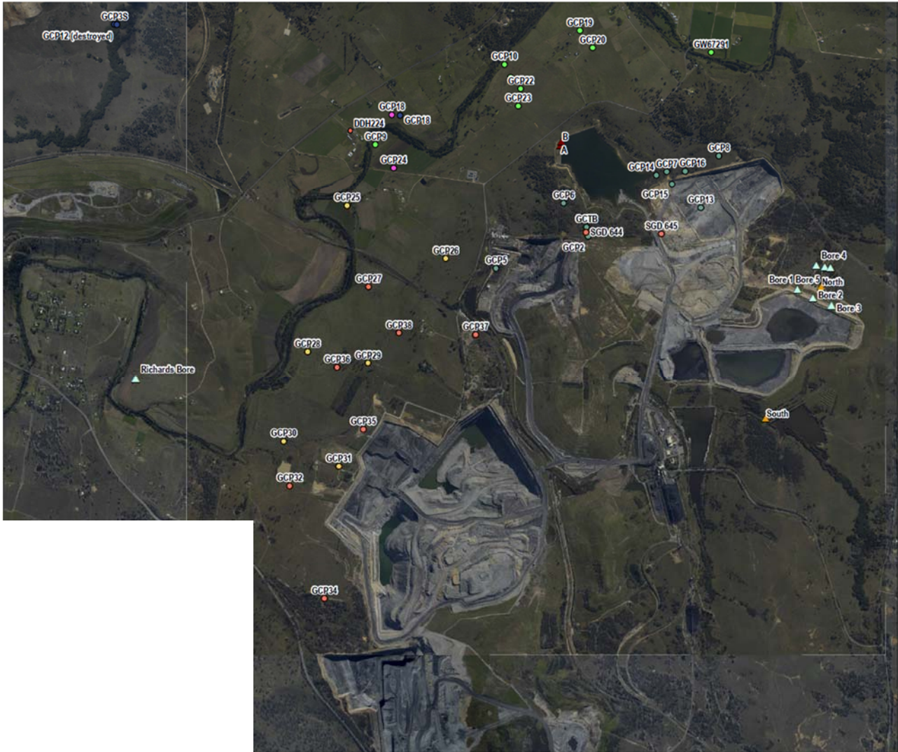
Figure 28 Rix’s Creek North Ground Water Monitoring Network
