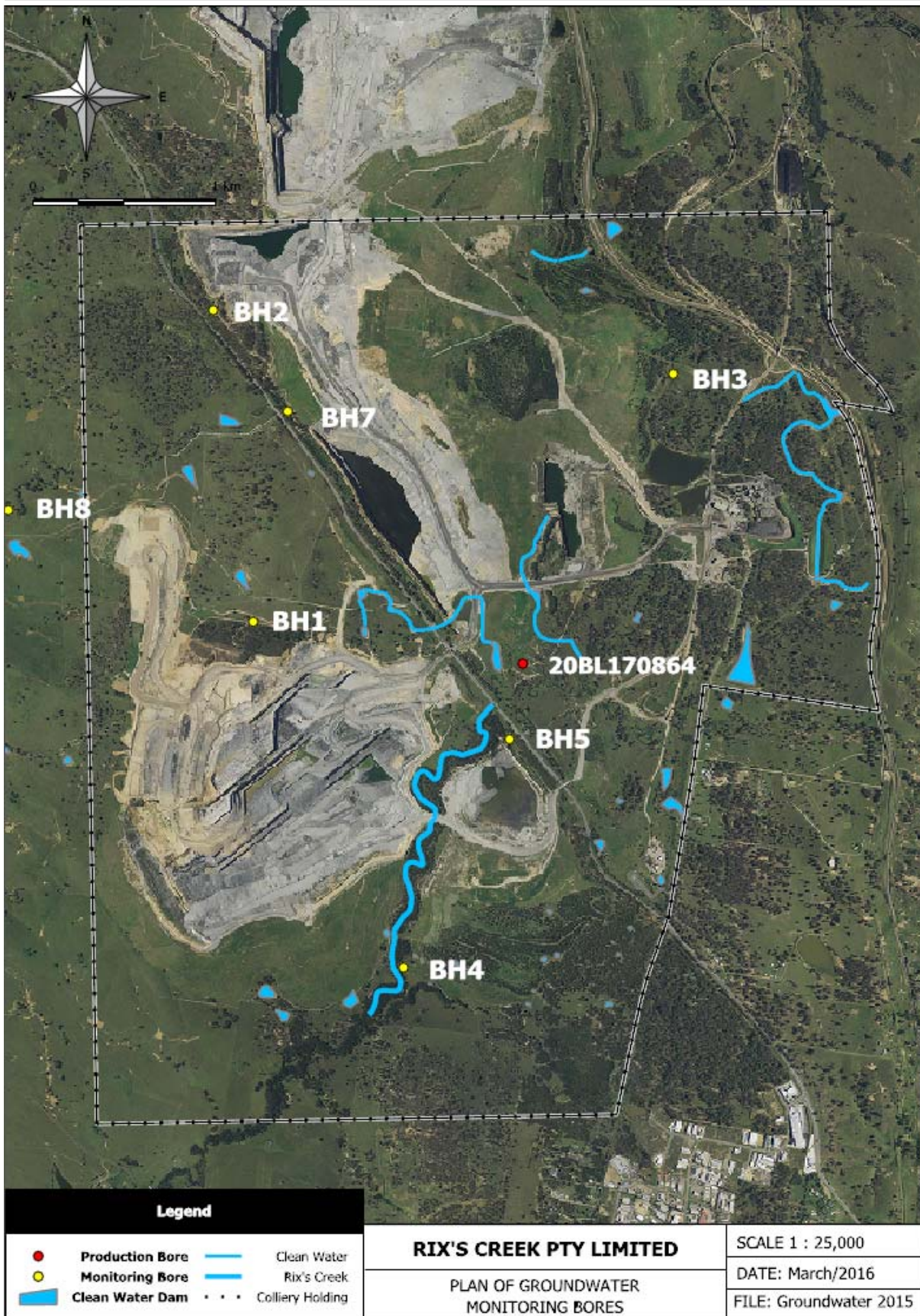
Figure 29 Rix's Creek South Groundwater Monitoring Network
